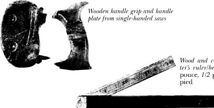
Wood and copper-alloy carpenter's ruler/bevel marked in 1/4 pouce, 1/2 pouce, pouce, and pied
